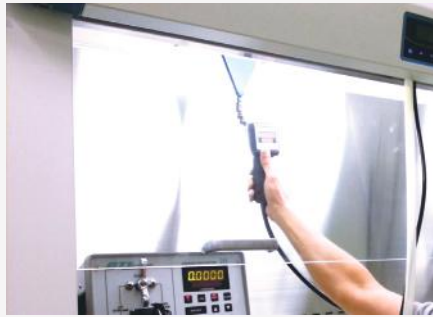
HEPA Filter Leak Test
